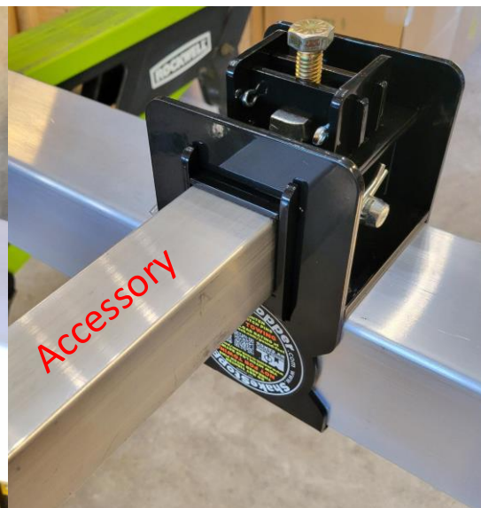
9. Insert Accessory into Hitch, tighten Pressure Bolt until no movement, then torque Carriage Bolt Locknut to firmly clamp Hitch to Bumper. Loosen Pressure Bolt to remove accessory. Hitch is now ready to use!
