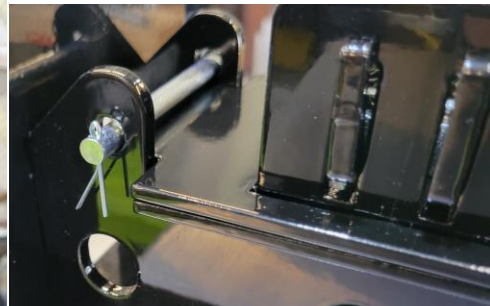
8. Insert Retention Pin through Side Plates, then insert/expand small Cotter Pin.
