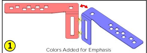
STEP 1: Separate UPPER and LOWER BRACKETS by Working Pieces Back and Forth as Shown. NOTE: Either Bracket can be UPPER or LOWER BRACKET Depending on Orientation of SUPPORT ARM.
