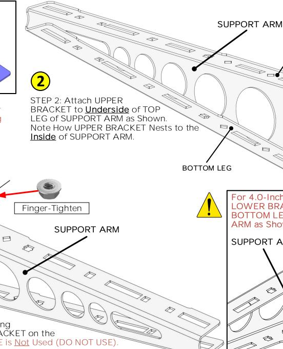
STEP 3: Attach LOWER BRACKET to SUPPORT ARM using LOWER SIDE HOLE with VERTICAL LEG of LOWER BRACKET on the Outside of SUPPORT ARM as Shown. UPPER SIDE HOLE is Not Used (DO NOT USE)
