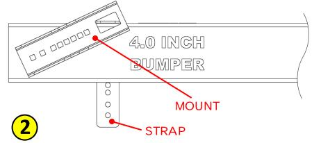
Insert STRAP Into MOUNT Rotate MOUNT as shown so as to insert STRAP through rectangular hole.
